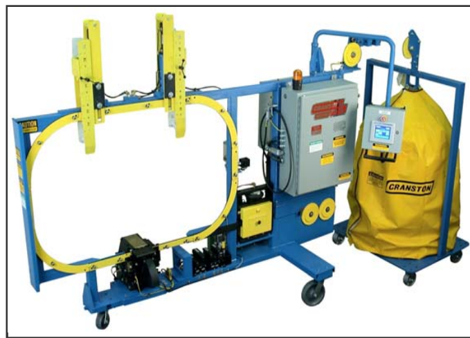
Series 987EP Wire Strapping Machine applies wire.
