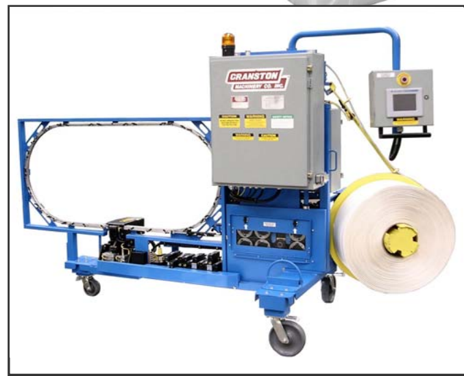
Rap Strap Machine, applies "Rap Strap" repulpable paper strapping.
