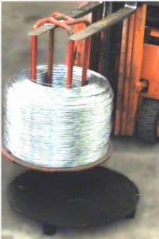
Loading a full wire stand onto the steel pallet can be accomplished by forks, or overhead hoist
